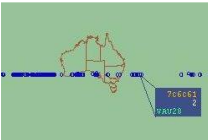
Figure 1 - Track Jumping problem with TPR901
